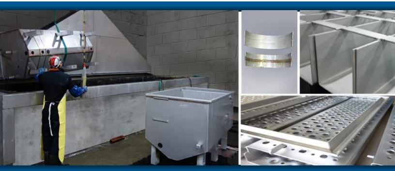
Pickle Passivation is the immersion of metal in a pickling bath or coating with nitric-hydroflouric acid. Pickle passivated stainless material has a light matte appearance. Customers use Apache's in house passivation services for:
